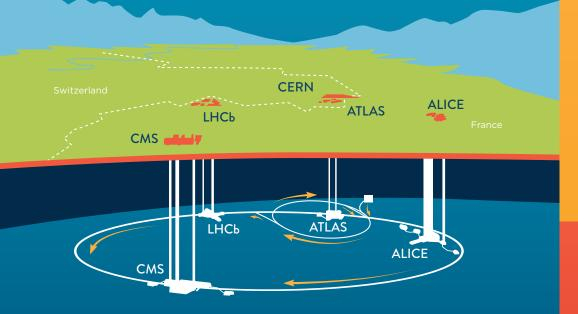
Proton beams are circulated in both directions around the LHC's 27km circumference ring and are brought into collision at four points, approximately 100m below ground. The LHCb experiment is located at one of these points and is the LHC experiment dedicated primarily to looking for differences between matter and antimatter in particles containing beauty and charm quarks. The UK is the lead contributing nation to the LHCb experiment.
